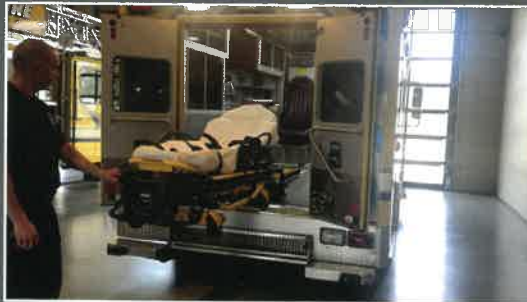
Vandalia's medic vehicles are now equipped with cot lifting devices, which make it much easier and much safer to place patients in the back of the vehicle.
