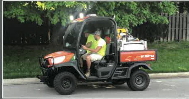
(Above) The Public Works Department purchased a utility vehicle with a mounted spray tank to eliminate vegetation in the roadways, curbs and gutters.
